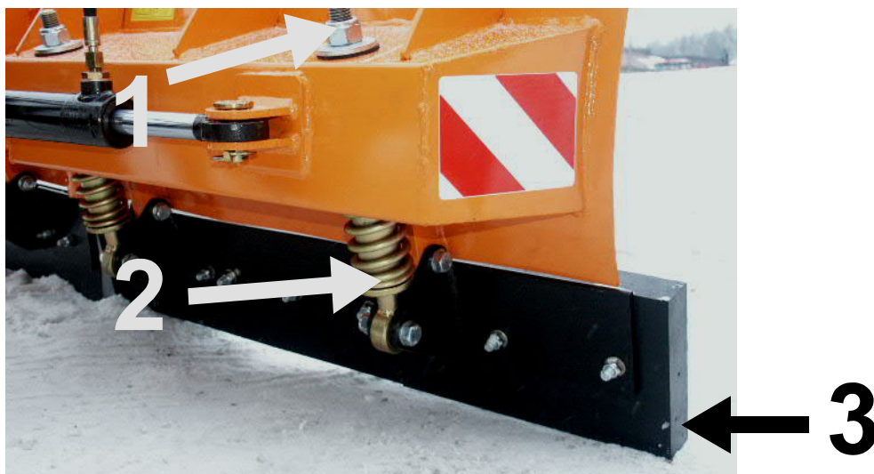
Fig. 9 Adjustment of inclination of scrapping slats
